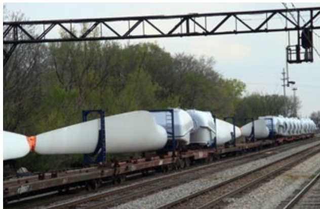
Wind turbine blades transported by train 86
